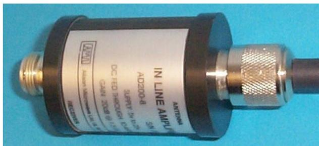
*T-AD200-8 GPS in-line amplifier 20dB*
